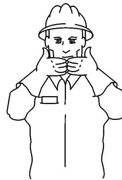
ALL DONE CLEAN-UP
